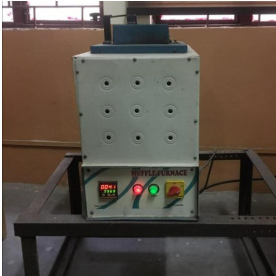
Figure15: Muffle Furnace during Sintering Process
