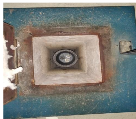
Figure 14: Placing samples inside the furnace.
