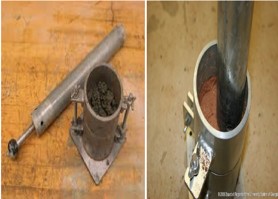
[ Figure 3.8 Proctor Compaction Test, Source:Google ]
