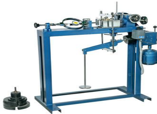
[ Figure 3.9 Direct Shear test Apparatus, Source:Google ]
