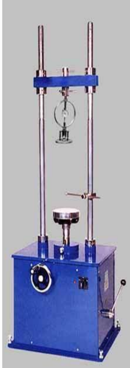
[ Figure 3.11 unconfined compressive strength Apparatus, Source:Google ]
