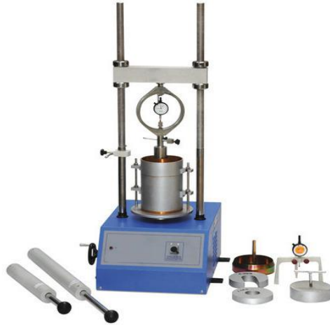
[ Figure 3.12 California Bearing Ratio CBR Apparatus, Source:Google ]
